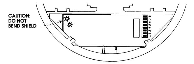
Switches 1 and 2 set the HOUSE CODE; 3-5 the first digit of the SENSOR NUMBER; and 6-8 the second digit of the SENSOR NUMBER.
